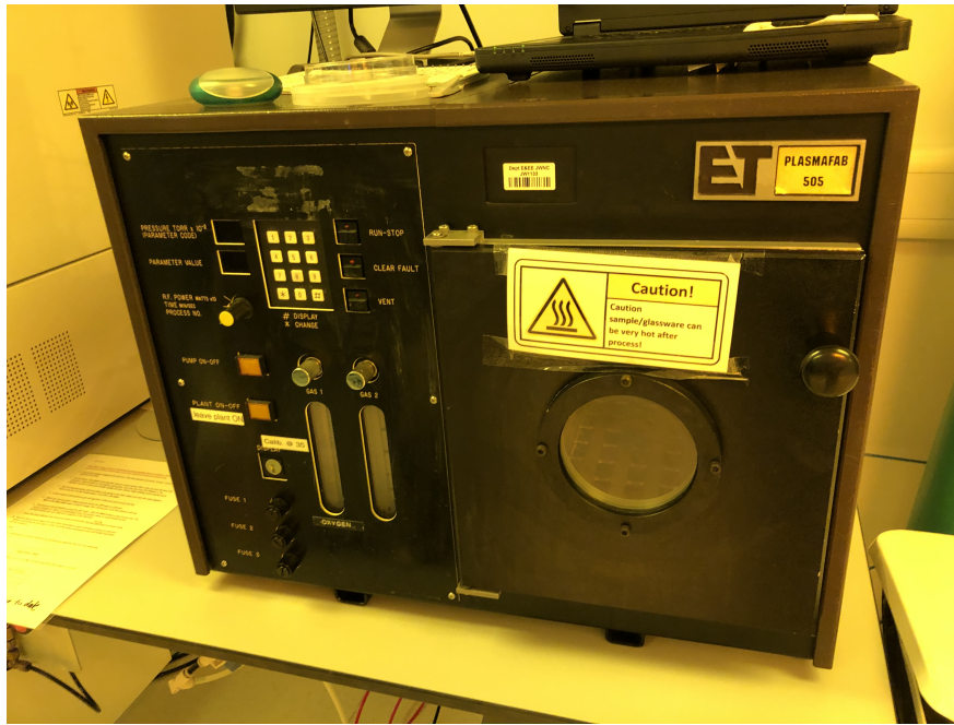
Figure 3.13: Plasmafab 505 Barrel Asher used to expose PDMS and glass substrate.
