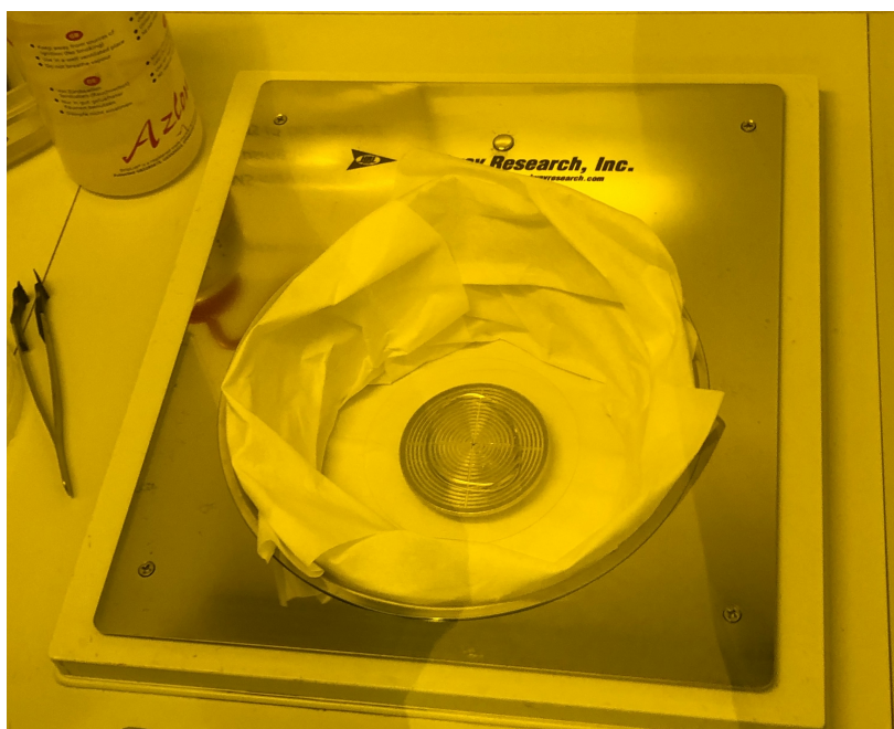
Figure 3.9: Spinner with SU-8 3050 deposited on working surface prior to spinning.
